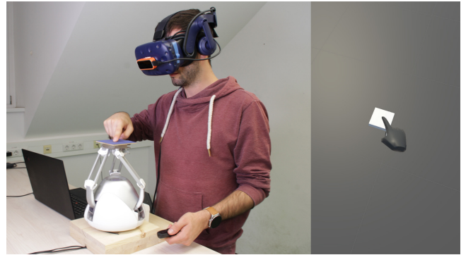
Figure 2: The experimental setup consists of the Novint Falcon haptic device with a custom-built end-effector, a Head-Mounted Display with an attached Leap Motion Controller to track participants' hands, a Gaming Laptop running the virtual environment, and a wireless presenter for participants to give their answers. Participants pressed down on the center of the provided touchable surface with their index fingers to displace the end-effector.
